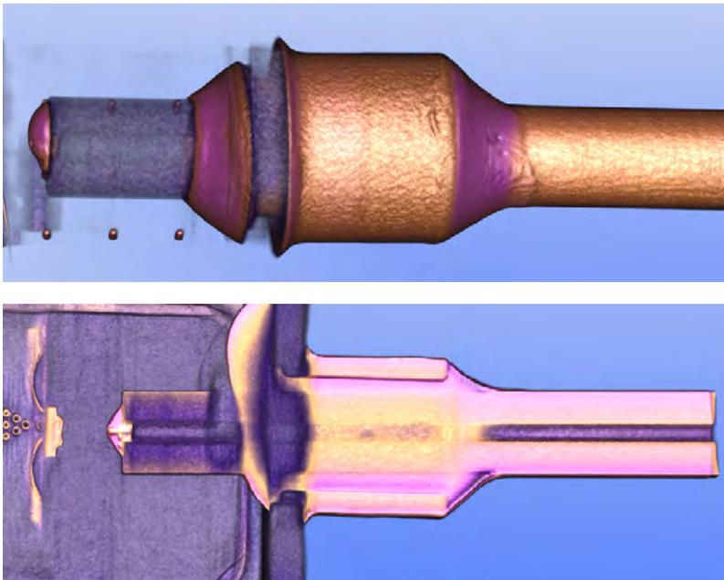
*Computerised Tomography X-ray images showing fibre feed-through of a photodiode component*
